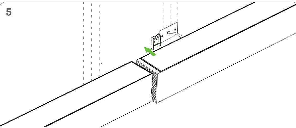
**FOR A CONTINUOUS ROW SYSTEMS:** WITH FIRST FIXTURE IN PLACE, REPEAT STEPS **2** AND **4**
