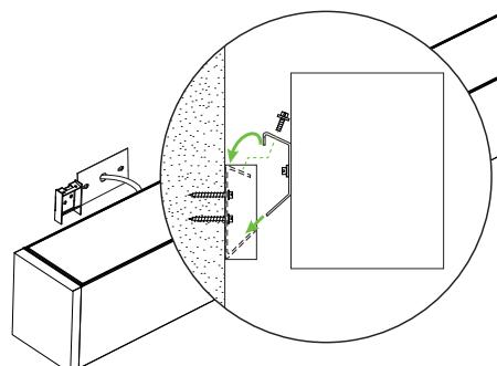
FASTEN THE FIXTURE BRACKET INTO THE WALL BRACKET AND SECURE WITH SUPPLIED WALL BRACKET SCREWS
