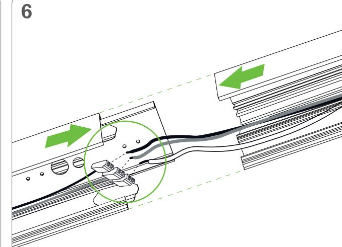
**FOR A CONTINUOUS ROW SYSTEMS:** WITH FIRST FIXTURE IN PLACE, REPEAT STEPS 1 AND 4 FOR THE NEXT FIXTURE IN LINE
