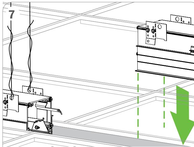
REPEAT STEPS ① AND ② FOR THE SECOND FIXTURE. ENSURE THAT SAFETY BRACKETS SIT ABOVE THE T-BARS.
