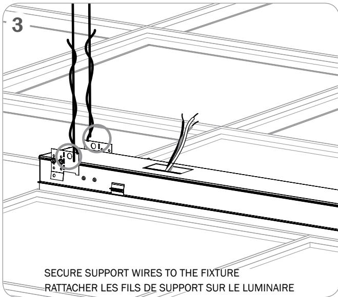
SECURE SUPPORT WIRES TO THE FIXTURE
