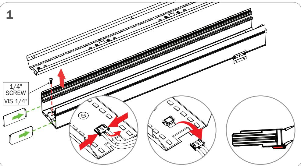
REMOVE 1/4" SCREW AND LED CARTRIDGE. UNPLUG BOARD CONNECTOR BY SQUEEZING SIDE ARMS AND LIGHTLY LIFTING BACK OF CONNECTOR TO CLEAR RECTANGLE IN BOARD. SLIDE IN 2 ALIGNER SPLINES
