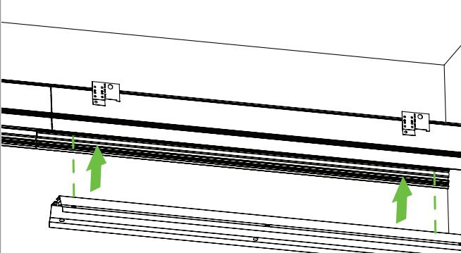
PLUG CONNECTOR HARNESS INTO LED BOARD AND INSTALL LED CARTRIDGE
