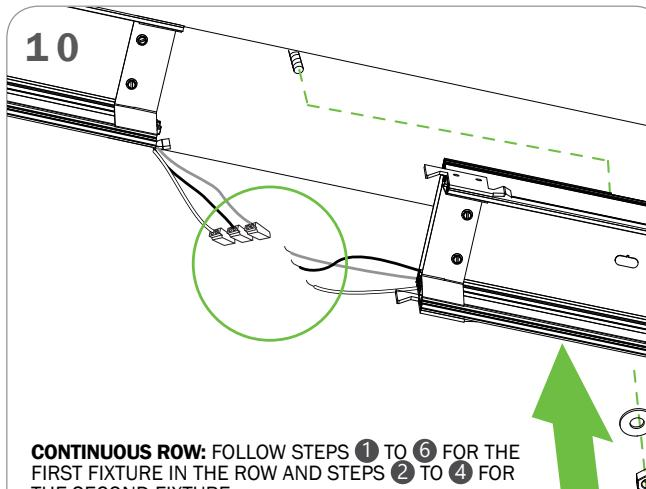
**CONTINUOUS ROW:** FOLLOW STEPS ① TO ⑥ FOR THE FIRST FIXTURE IN THE ROW AND STEPS ② TO ④ FOR THE SECOND FIXTURE
