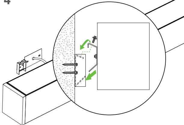
FASTEN THE FIXTURE BRACKET INTO THE WALL BRACKET AND
