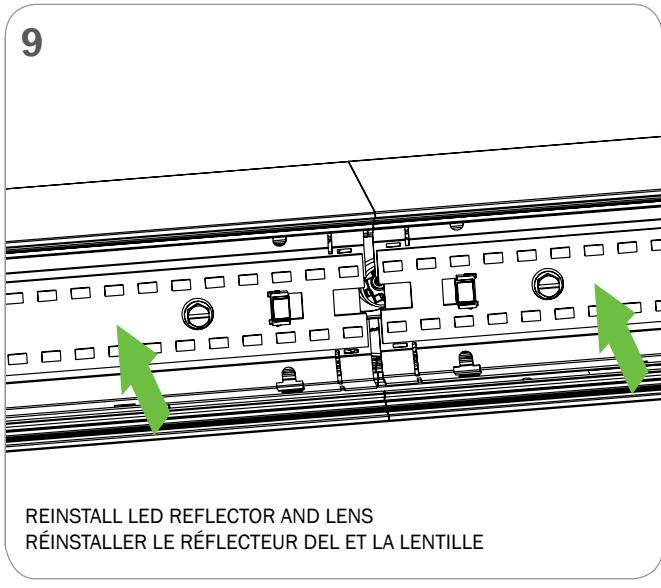
REINSTALL LED REFLECTOR AND LENS
