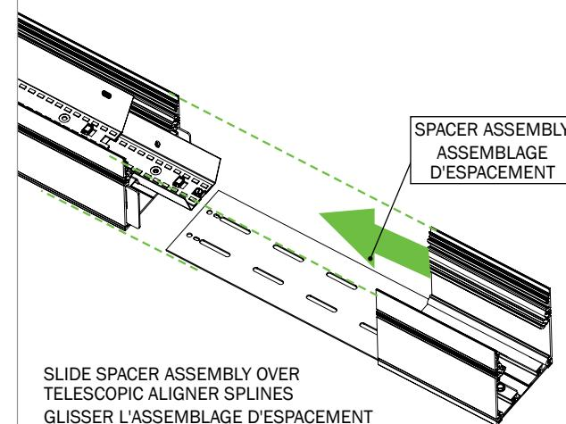
SLIDE SPACER ASSEMBLY OVER
