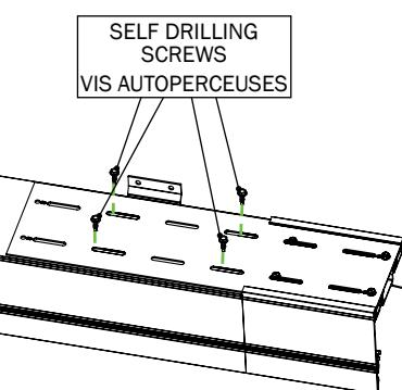
PLACE SPACER ASSEMBLY OVER EXTRUSION AND SECURE
