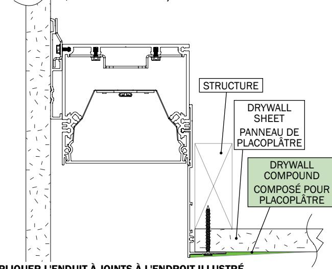
**APPLY DRYWALL COMPOUND AT AREA SHOWN / APPLIQUER L'ENDUIT À JOINTS À L'ENDROIT ILLUSTRE**
