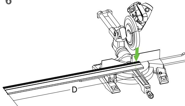
CUT SIDE EXTRUSION TO MATCH TOTAL LENGTH "D" OF
