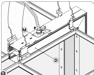
Secure Knockout plate (M) to the lit corner section (D) by fastening a screw.
