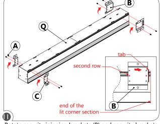
Rotate security joinning brackets (B) and security brackets (C) 90 degrees. Using screws (A) from step place safety joining brackets (B) and security brackets (C) back to the ceiling straight section (Q) using second row of holes, place the tab of the security joinning brackets (B) flush to the end of the straigt section (Q).
