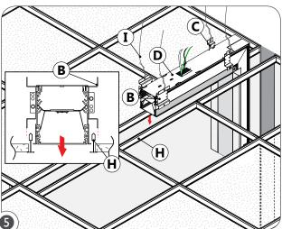
Lower the inside lit corner section (D) onto the T-bar runner (H). Ensure that the safety joining brackets (B) and security brackets (C) sit above the T-bars (H). For additional safety, a security wire (I) can be attached onto the safety joinning brackets (B) and security brackets (C) to the structure above.
