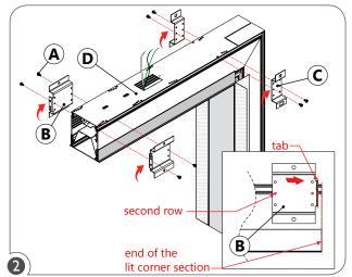
Rotate security joinning brackets (B) and security brackets (C) 90 degrees. Using screws (A) from step 1 place safety joining brackets (B) and security brackets (C) back to the inside lit corner section (D) using second row of holes, place the tab of the security joinning brackets (B) flush to the end of the sinside lit corner section (D).
