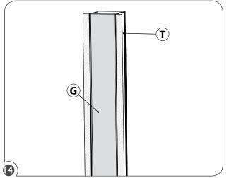
FOR NEXT VERTICAL WALL SECTION: Leave optic lens and blue tape (G) installed on the vertical wall section (T).
