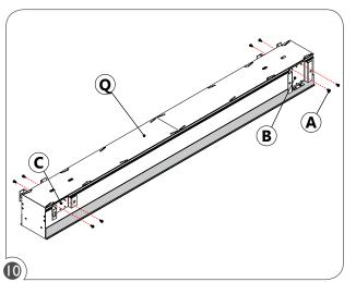
FOR NEXT CEILING SECTION: Remove screws (A) from the safety joining brackets (B) and security brackets (C) from the ceiling straight section (Q).
