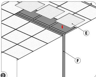
Remove ceiling tiles (E) where the fixture will be installed and adjacent tiles for easy access. Cut hole (F) in drywall according to the dimensions on the fixture shop drawing.
