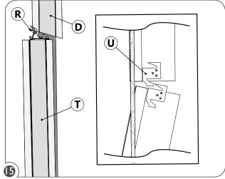
Make wire connections with guick-wire connectors (R) and slide the 2 sections together. Hook the brackets (U) together to join sections.
