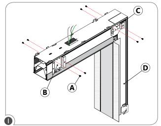
Ensure that the power to the fixture's circuit is turned off. Remove screws (A) from the safety joining brackets (B) and security brackets (C) from the inside lit corner section (D).
