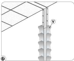
Plaster and sand over spackle flange (V) and drywall screws to create a smooth finish.
