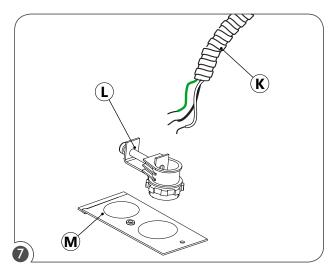
Pass the BX cable (K) into the BX cable connector (L). Install BX cable connector (L) onto the knckout plate (M).
