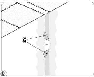
Remove blue tape (G) from optics lens before last plaster layer is fully dry.
