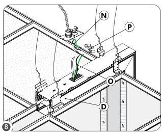
Connect BX cable wires (N) to the lit corner section (D) driver wires (O) using wire nuts (P).
