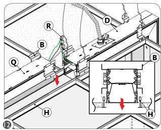
Lower the ceiling straight section (Q) onto the T-bar runner (H). Ensure that the safety joinning Brackets (B) and security brackets (C) sit above the T-bars (H). Make wire connection between ceiling straight section (Q) and Lit corner section (D) using The quick-wire connectors (R).
