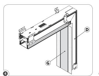
When installing inside lit corner section (D), leave the blue tape (G) on the optic lens to prevent damage. Leave optic lens installed on the inside lit corner section (D).
