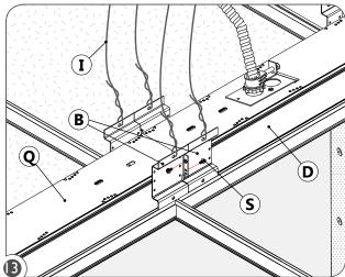
Secure the sections together, by screwing the security joinning brackets (B) to each other with provided screws (S). For additional safety, a security wire (I) can be attached onto the safety joinning brackets (B) and security brackets (C), on the ceiling straight section (Q), to the structure above. Ceiling tiles (E) can be placed back into their position.
