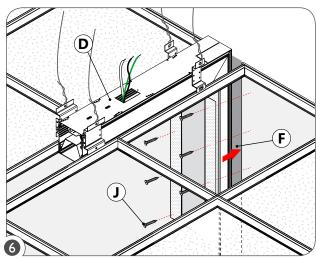
Push inside lit corner section (D) into hole in drywall (F) and fasten to the wall using drywall screws (J). If optic lens appears bowed or too loose, remove drywall screws (H) on one side of the section, adjust the section so that the lens fits flat and snug, and re-install screws.
