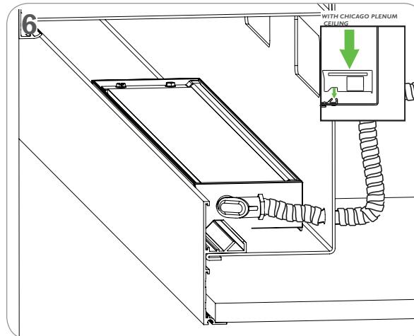
**CONTINUOUS ROW:** CONNECT BX-CABLE OF EACH FIXTURE TO MAIN STREAM IN ACCORDANCE WITH NATIONAL AND LOCAL BUILDING CODES
