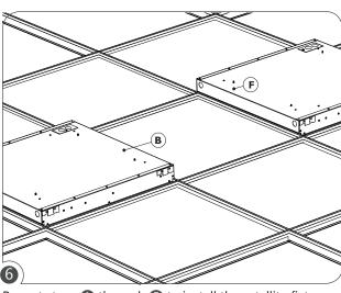
Repeat steps 1 through 5 to install the satellite fixture (F) adjacent to the master fixture (B).
