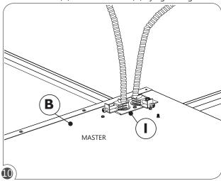
Push connected wires and wire nuts into master fixture (B). Reinstall knockout plate (I) onto fixture by hooking tab into hole, and refastening screw to knockout plate and housing.
