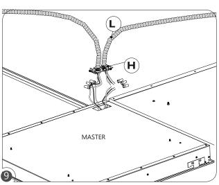
Insert satellite BX cable (L) into BX connector (H) and fasten by tightening screw. Connect satellite BX cable (L) wires to wires labeled for satellite inside the fixture. A wiring diagram is also provided.
