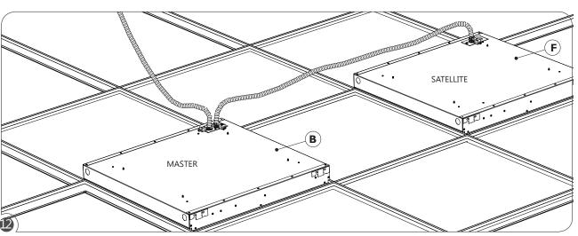
Make sure that proper alignment is maintained and all fixtures are correctly oriented in relation to other fixtures.
