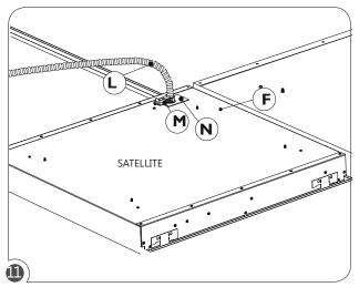
Remove knockout plate (N) from satellite fixture (F), and connect satellite BX cable (L) to satellite BX connector (M). Connect satellite BX cable wires to wires in satellite fixture. Reinstall knockout plate (N) on satellite fixture (F).
