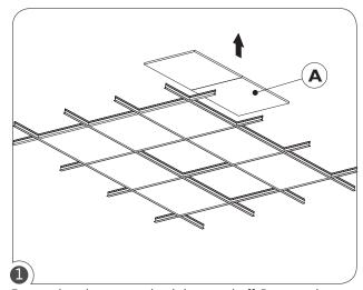
Ensure that the power circuit is turned off. Remove the ceiling tiles (A) where the fixtures will be installed and adjacent tiles for easy access when connecting the wires.
