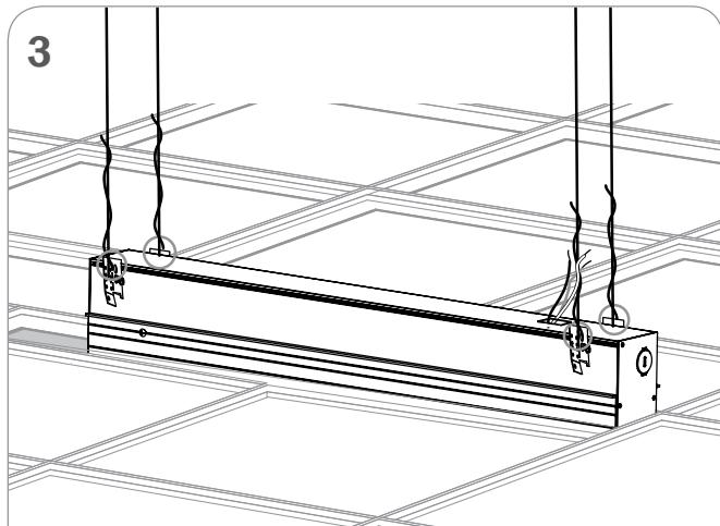
SECURE SUPPORT WIRES TO THE FIXTURE
