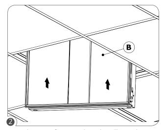
Insert the master fixture (B) above the ceiling as shown.
