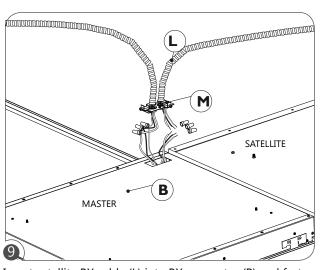
Insert satellite BX cable (L) into BX connector (P) and fasten by tightening screw. Connect satellite BX cable (L) wires to wires labeled for satellite inside the master fixture (B). A wiring diagram is also provided.
