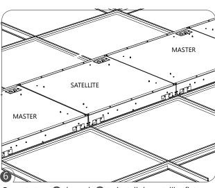
Repeat steps 1 through 5 to install the satellite fixture (I) next to the master fixture (A).
