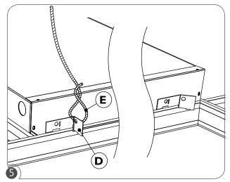
For additional safety a security wire (E) can be attached from the T-bar tabs (D) to the structure above.
