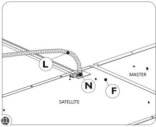
Remove knockout plate (N) from satellite fixture (F), and connect satellite BX cable (L). Connect satellite BX cable (L) wires to wires in satellite fixture (F). Reinstall knockout plate (NQ) on satellite fixture (F).
