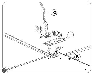
Remove knockout plate (I) from the top of the master fixture (B) and install BX connector (H) through the knockout plate (I). Insert the power feed BX cable (G) into BX connector (H), and fasten BX cable (G) to BX connector (H) by tightening screw.
