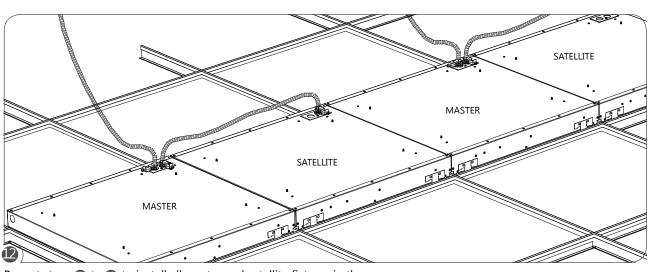
Repeat steps **1** to **1** to install all master and satellite fixtures in the row. Make sure that proper alignment is maintained and all fixtures are correctly oriented in relation to other fixtures.
