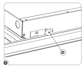
Based on ceiling type (tegular / screw slot T-bar or standard T-bar) bend a tab (D) on each corner of the fixture to provide support. (SEE T-BAR STYLE MOUNTING GRAPHIC).
