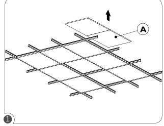
Remove the ceiling tiles (A) where the fixtures will be installed and adjacent tiles for easy access when connecting the wires.
