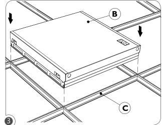
Set the master fixture (B) into the T-bar grid (C).
