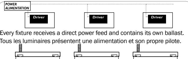
Every fixture receives a direct power feed and contains its own ballast.
