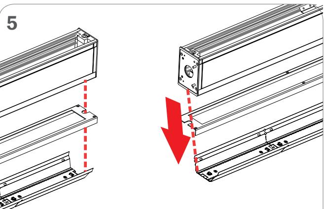
**SYSTEM RUN:** REPEAT STEPS 1 TO 4 FOR THE NEXT FIXTURE IN LINE
