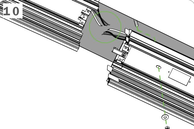
**CONTINUOUS ROW: FOLLOW STEPS ① TO ⑥ FOR THE FIRST FIXTURE IN THE ROW AND STEPS ② TO ④ FOR THE SECOND FIXTURE**
