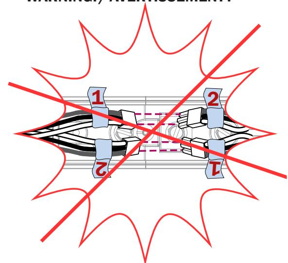
**ENSURE NO WIRES ARE IN THE WAY WHEN SNAPPING ON COVER**
