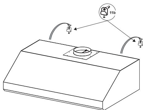
Hook the hood body onto the wall plugs.
