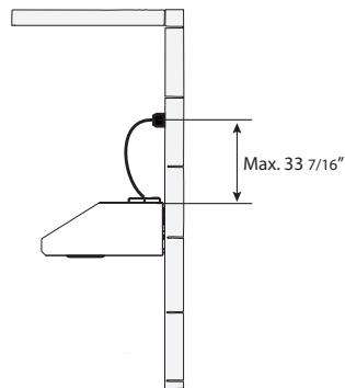
The supply cord shall be accessible for inspection after installation.
