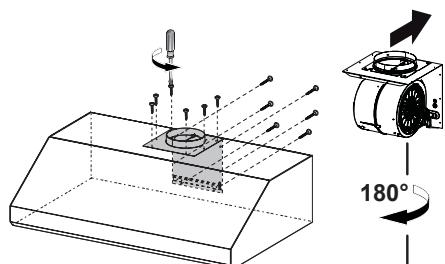
For a horizontal ducting installation the motor needs to be unsecured by first removing the 12 screws as shown.
