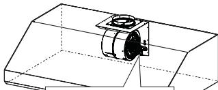
**⚠** The Electrical Connector must be removed first before converting the hood to Rear Ducting mode.
