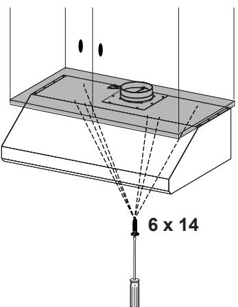
Fix the Hood Body with 4 screws from the bottom.
