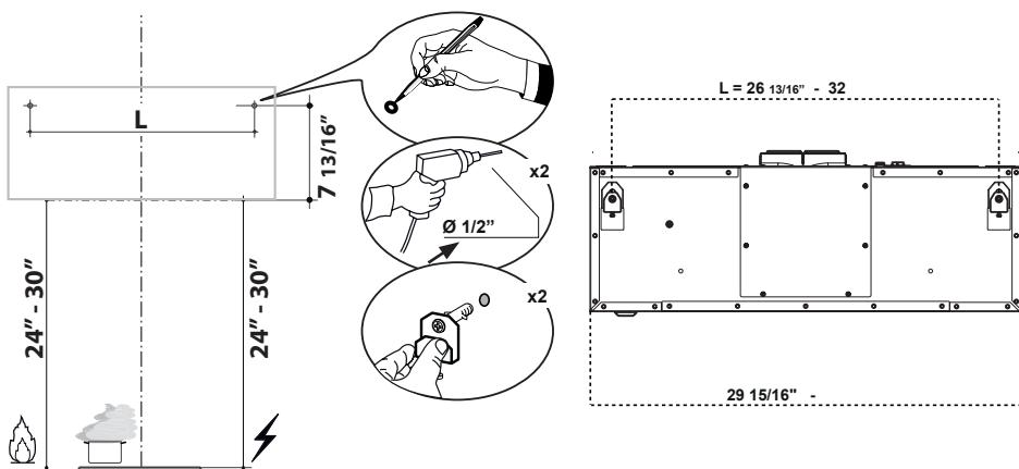
Mark the wall where indicated,  $7 \frac{13}{16}"$  above the horizontal line and at L distance on the left and right of vertical line. The distance L change for all dimension of Hood.
