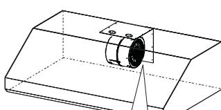
Once the blower is in place re-install the 12 screws to fasten the motor to the Hood body.
