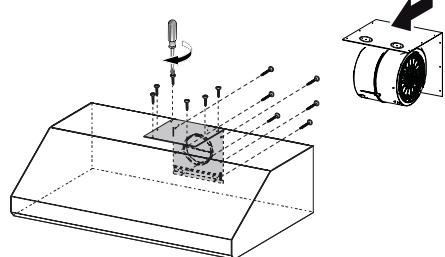
Once the screws are removed, extract the blower from the body of the Hood and position it so the transition opening is facing to the rear wall (from the back remove and rotate 180 degrees to the left, and then flip it back 90 degrees as shown in the diagram).
