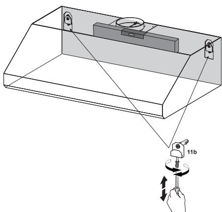
Use a level to insure that Fixing Bracket is level and then fully secure the two screws.
