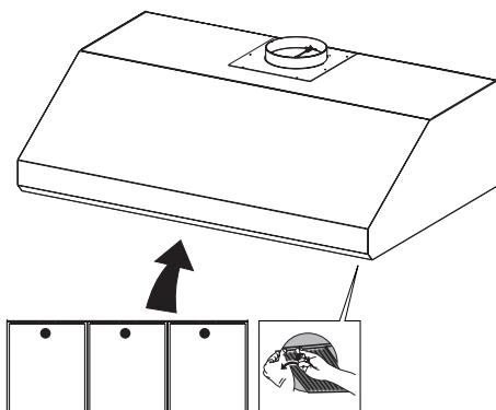
Replace the filters removed previously.
