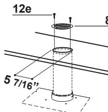
For Non-Ducted Recirculation venting route the ductwork to a location above the hood where the discharge is vented back into the room.
