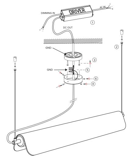
Note: Line voltage must be installed by a qualified electrician, in accordance with local electrical laws.
