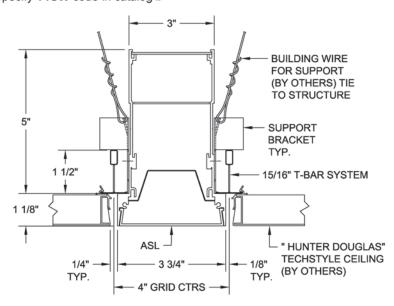
Mounting bracket is field adjustable to accommodate both conditions.
