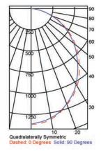
Fixture with T8 lamping (One lamp using Standard Diffuse lens. For Medium and Heavy diffuse lenses, use multiplier on page 2.)
