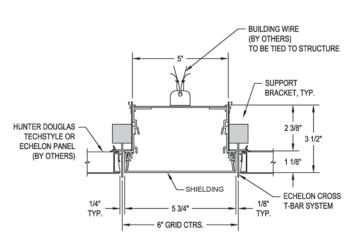
Mounting bracket is field adjustable to accommodate all four conditions.
