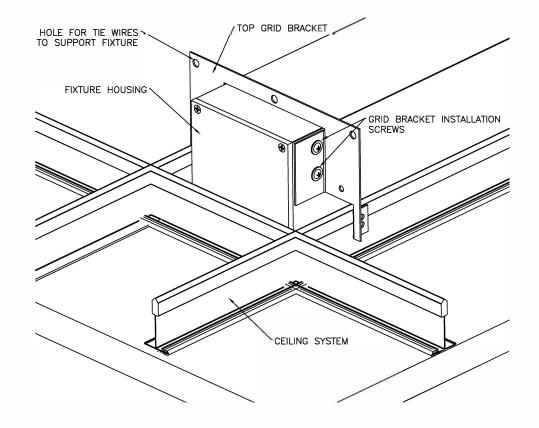
REMOVAL OF THE TOP GRID BRACKETS BY INSTALLING CONTRACTOR IS NECESSARY TO RAISE FIXTURES INTO THE CEILING SYSTEM. ONCE IN THE GRID, CONTRACTOR TO REINSTALL THE TOP GRID BRACKETS. ACCESS TO UPPER CEILING STRUCTURE IS REQUIRED TO MOUNT THE FIXTURES.
