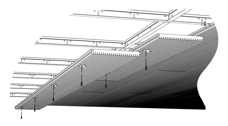
The 3100 Acoustic Plank wood ceiling offers a design with fine linear grooves. Typical planks are 192 mm (7 9/16") wide, with 1/16" wide grooves spaced 8mm (5/16") or 16mm (5/8") on center. Due to required fabrication tolerances, only engineered veneered wood composites are used. Member lengths are 8' to maximize yield of veneered sheet goods.
