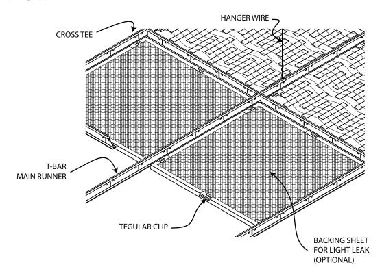
The 3200 Acoustic Tile wood ceiling offers a design with tiles consisting of fine linear grooves assembled from acoustic planks. Typical Acoustic Tiles are 24" x 24", 24" x 48" and 48" x 48". Grooves are 1/16" wide, spaced 8mm (5/16"), 16mm (5/8"), or 32mm (1 1/4") on center. Due to required fabrication tolerances for Acoustic Tile, engineered veneered wood composites must be used.
