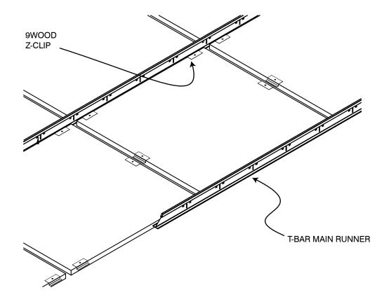
The 4100 Tegular Tile wood ceiling offers a tiled appearance. The 4100 Tegular Tile hangs from and is accented by 9/16" standard black T-Grid. Reveals between panels are created by the width of the T-Bar flange (i.e., 9/16").
