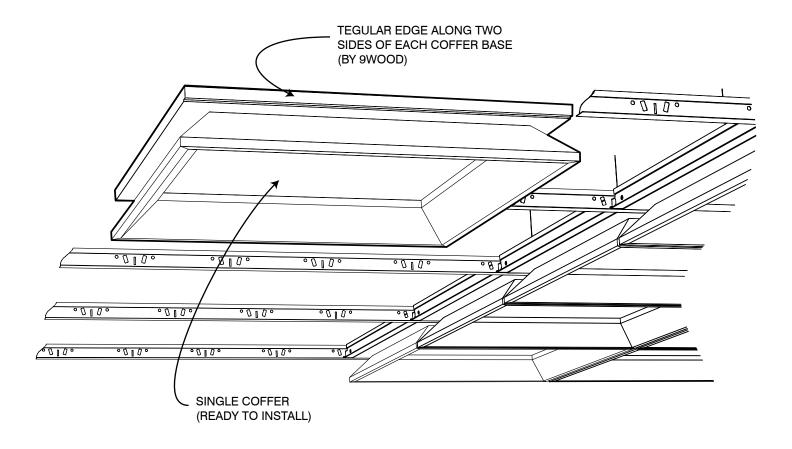
The 7200 Modern Molding Coffer style wood ceiling offers a coffer design typical of modern European woodwork. The coffer frame remains angular. The coffer lays into 15/16" standard T-Bar grid below the grid. Multiple veneer pattern options are available for the coffer interior panel.
