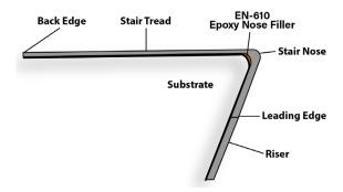
Overlap the stair tread above the riser with the riser while ensuring that riser toe is not over-compressed. Using the leading edge of the stair tread as a guide, use a divider or a marking tool to scribe the riser. Use a suitable knife to trim riser along the scribe mark.
