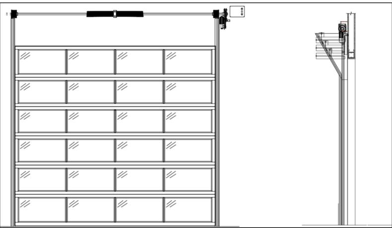
The Sovereign system is balanced by the use of torsion springs connected to a rotating shaft. The shaft ends are attached to cable drums that lift / lower the curtain, and no overhead tracks.
