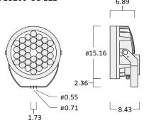
1. Prior to electrical connection, proceed with mechanical installation by firmly fixing yoke A to optional mounting accessory or directly to a suitable surface.
