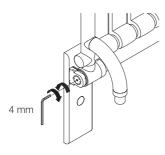
Clockwise: increase braking force Counter-clockwise: reduce braking force
