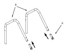
Slide Front Legs onto Back Frame (C). Fasten using 4 Small Assembly Screws and Fasteners.
