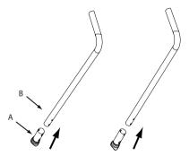
Slide Handles onto Back Frame and fasten with 4 Small Assembly Screws and Fasteners. Slip Grips (C) onto Handles.
