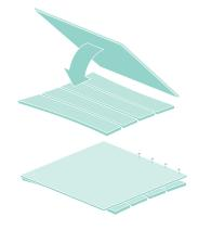
Due to expansion/contraction of individual boards during seasonal changes a 1/4" or thicker APA underlayment panel must be installed over these types of subfloors.
