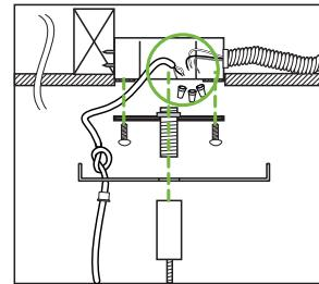
Example of a junction box in a ceiling (Installation sheets for all mounting options are available at: [www.axislighting.com](http://www.axislighting.com)).
