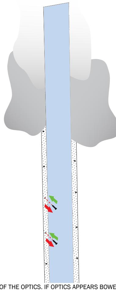
CHECK THE FIT OF THE OPTICS. IF OPTICS APPEARS BOWED OR TOO LOOSE, REMOVE SCREWS ON ONE SIDE OF THE FIXTURE, ADJUST THE FIXTURE AND RE-INSTALL SCREWS. PLASTER AND SAND OVER SPACKLE FLANGE.
