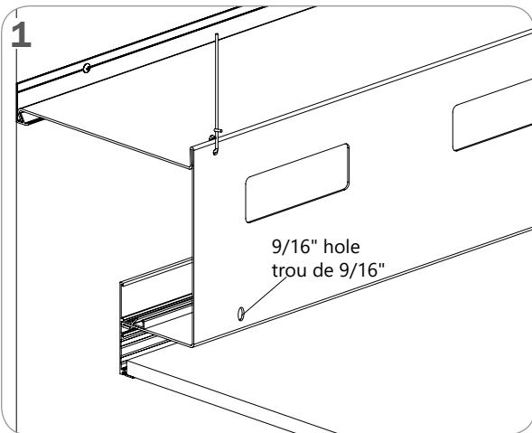
Make a 9/16" hole in ceiling cove to pass T-connector.
