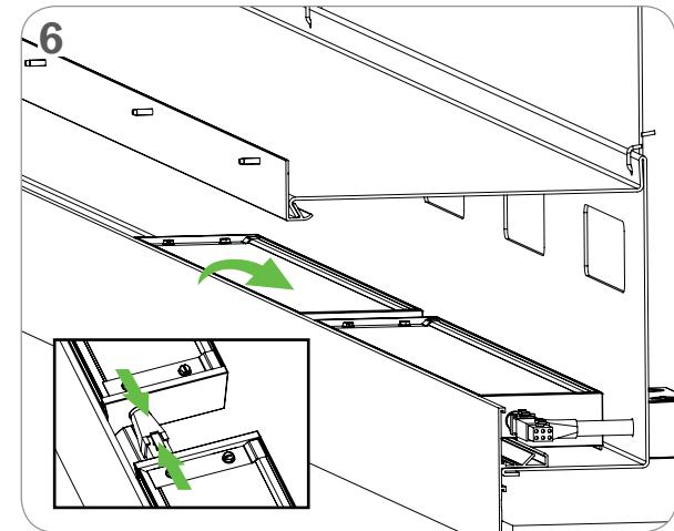
**CONTINUOUS ROW:** CONTINUE PLACING FIXTURES IN CEILING COVE AND CONNECTING TO PREVIOUS FIXTURES UNTIL FINISH OR MAXIMUM CIRCUIT AMPERAGE IS REACHED
