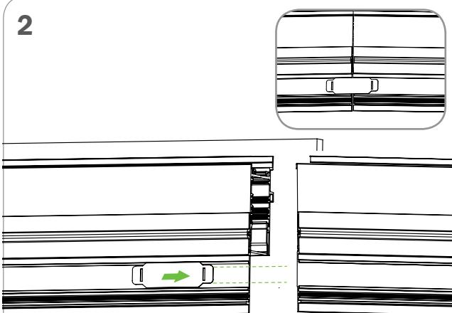
**CONTINUOUS RUN:** INSTALL ALIGNER INTO THE FIRST EXTRUSION. REPEAT STEPS 1 AND 2 FOR THE NEXT FIXTURE
