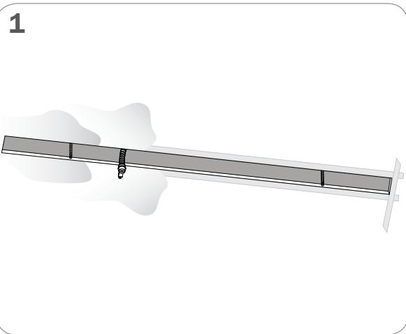
MAKE AN OPENING IN DRYWALL ACCORDING TO THE DIMENSIONS ON THE SHOP DRAWINGS
