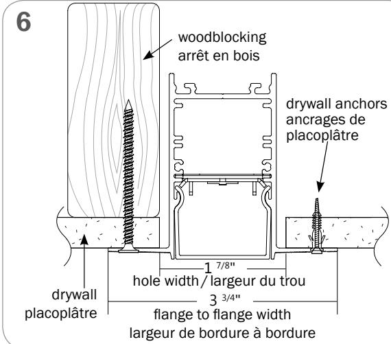
WOOD BLOCKING OR DRYWALL ANCHORS MUST BE USED TO REINFORCE THE SCREWS TO THE DRYWALL
