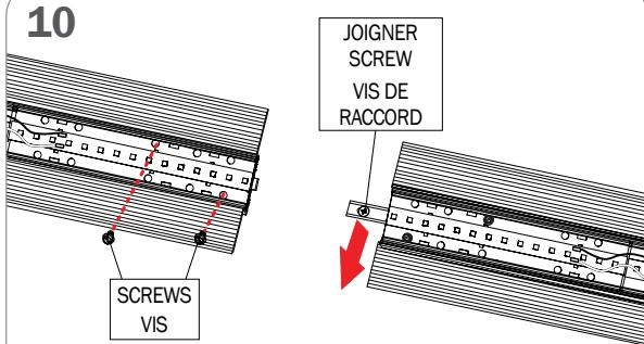
**CONTINUOUS ROW:** FOLLOW STEPS 1 TO 7 FOR FIRST FIXTURE IN CEILING, THEN: REMOVE SCREWS FROM LED BOARDS ON EXTREMITIES AND JOIGNER BRACKET
