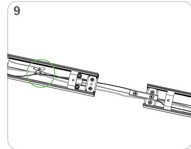
**CONTINUOUS ROW:** FOLLOW STEPS 1 TO 6 FOR FIRST FIXTURE AND 2 TO 4 TO INSTALL NEXT FIXTURE IN CEILING, THEN: CONNECT THE ELECTRICAL WIRES BETWEEN THE TWO FIXTURES
