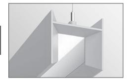
One-piece acrylic lens with **Microgroove Side Spotless** (MSO) side shielding.
