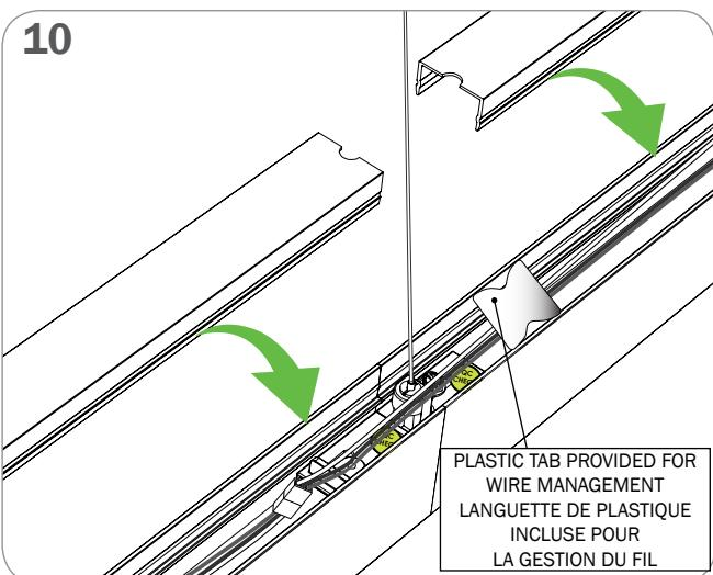
ENSURE NO WIRES ARE IN THE WAY WHEN SNAPPING ON COVER
