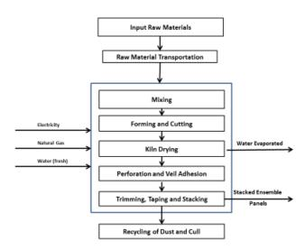
The manufacture of Ensemble<sup>™</sup> panels starts with the combining of the dry ingredients in a screw conveyor, feeding of this dry ingredient mixture into a pin mixer where these dry ingredients are mixed with water and wet additives. The resulting slurry is fed between two sheets of paper; facing paper (Manila) on the bottom and backing paper
