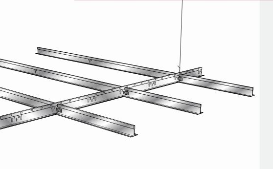
The base is a standard USG drywall suspension system.
