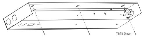
3. Access the wiring by removing (2) palnuts as shown and hinging the wireway down.
