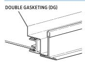
Gasketing is factory-installed continuously between door frame and luminaire housing; and between door frame and lens.
