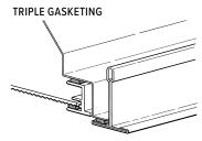
Gasketing is factory-installed continuously between door frame and luminaire housing; and between door frame and lens. Gasketing between bottom perimeter of unit (adjacent to T-bar or hardpan ceiling) is provided by factory and field installed.
