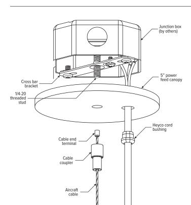
**STEP 1:** Mount the cross bar bracket to the junction box.
