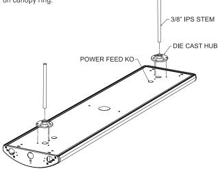
**Note:** Two stem sets required for 4' fixture; three stem sets for 8'. One additional stem set required for each 4' length when row mounted.
