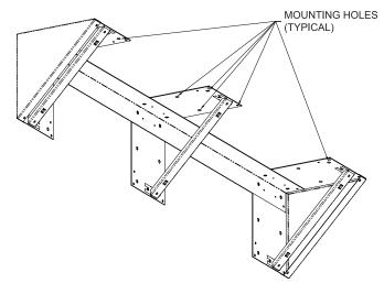
**9.** Position fixture over corner mounting bracket and secure with 1/4-20 screws (furnished). If row mounting, align, bolt, and fasten wiring harness per step 5 of these instructions. Finish electrical connections, reinstall the wireway cover, lamps, and lens.
