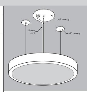
Note: ø5" canopy used at power feed location. Other suspension points use ø2" canopy.
