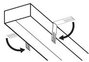
**STEP 4:** Hand bend outer tabs on the SRK brackets around the fixture housing sides to keep SRK brackets in the desired position.
