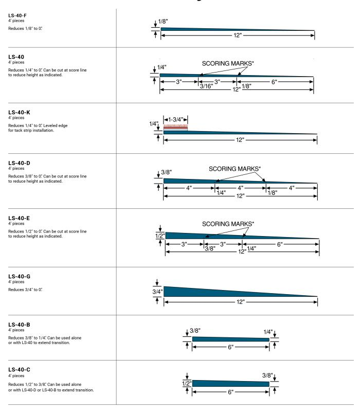
We've practically eliminated the need for traditional floor levelers—and the labor and curing time they require. Our patented SubFloor Leveler System® provides a gradual ramp between different flooring elevations, creating a smooth transition and fewer trips and falls. With easy installation and the ability to lay flooring immediately over top, it keeps everything moving swiftly—from your project to your foot traffic.
