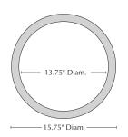
Materials: unsaturated polyester resin, sand, stone powder, talc powder, and fiberglass
